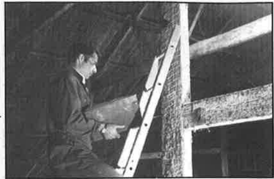
Peter Bannister collects wood samples from roof trusses in Pan House No.3
