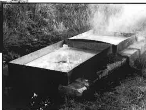
Right: Stainless steel and lead salt pans over a wood fire.
